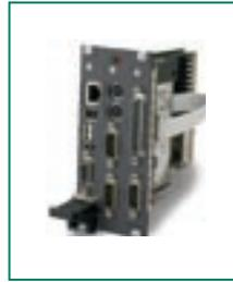
VFT *electronics* are in the form of plug-in modules that are inserted into an electronics cPCI chassis. Every VFT will have a **Master Control Unit (MCU)**. The MCU has a CPU, hard drive, two serial communication ports, multiple USB connectors, Ethernet connector, VGA connector and connectors for an external mouse and keyboard.
