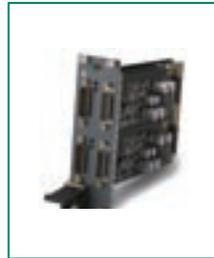
The **Test Control Unit (TCU)** is the core of the VFT's power and flexibility. Each TCU features a 1.36 GFlop RISC microprocessor. The TCU is available as a single-channel or a dual-channel module. Each channel can accept up to six sensor inputs with scan times as fast as 260 usec or resolutions as high as 24 bits. Each channel has up to eight discrete outputs, four discrete inputs and one analog output.
