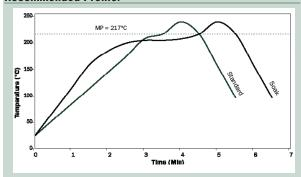
The stated profile recommendations apply to most Pb-free alloys in the SnAgCu (SAC) alloy system, including SAC 305 (96.5Sn/3.0Ag/0.5Cu). This can be used as a general guideline in establishing a reflow profile when using Indium8.9HF Solder Paste. Deviations from these recommendations are acceptable, and may be necessary, based on specific process requirements, including board size, thickness, and density.
